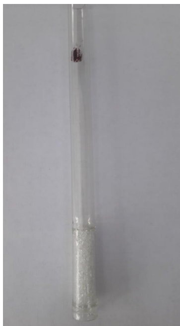
Fritted glass tube with reagents for active sampling
