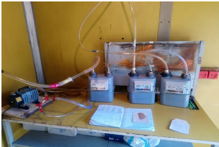
Air sampling system in Station N 1 in Yerevan
